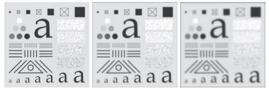
(a)A test pattern of size  $1024 \times 1024$ . (b) Result of lowpass filtering the pattern with a Gaussian kernel of size  $21 \times 21$ , with standard deviations  $\sigma = 3.5$ . (c) Result of using a kernel of size  $43 \times 43$ , with  $\sigma = 7$ . We used K = 1 in all cases.
