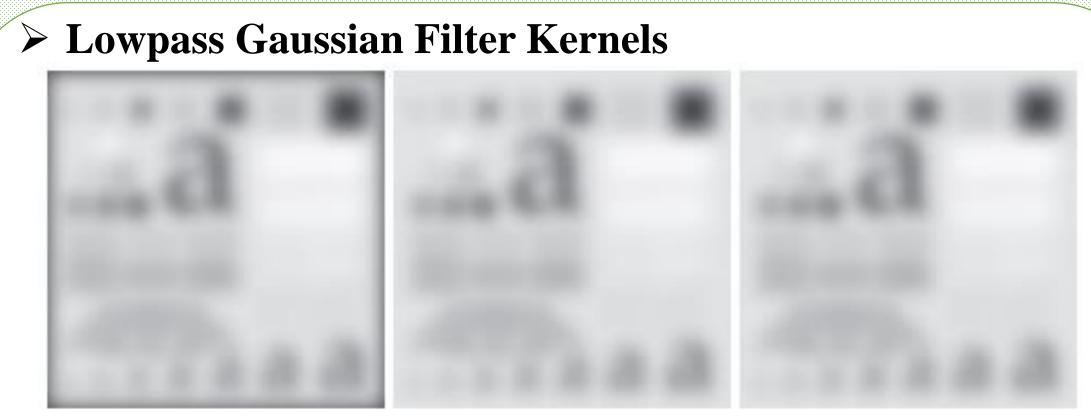
Result of filtering the test pattern in Fig. using (a) zero padding, (b) mirror padding, and (c) replicate padding. A Gaussian kernel of size  $187 \times 187$ , with K = 1 and  $\sigma$  = 31 was used in all three cases.
